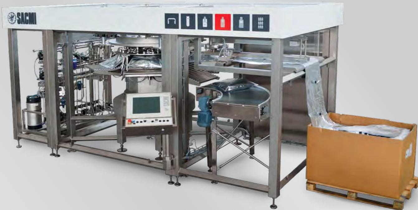
The filler is specially designed to automatically fill "pre-cut continuous module" or WEB type bags. Any type of spout may be used, even with a single guide spout, and may be placed in any position on the bag. A "size change over" kit is provided for each type of spout. All the most delicate operations that affect cap sterility such as uncapping, filling and capping take place in an aseptic chamber where the steady controlled flow of sterile air maintains a sterile environment at all times.
