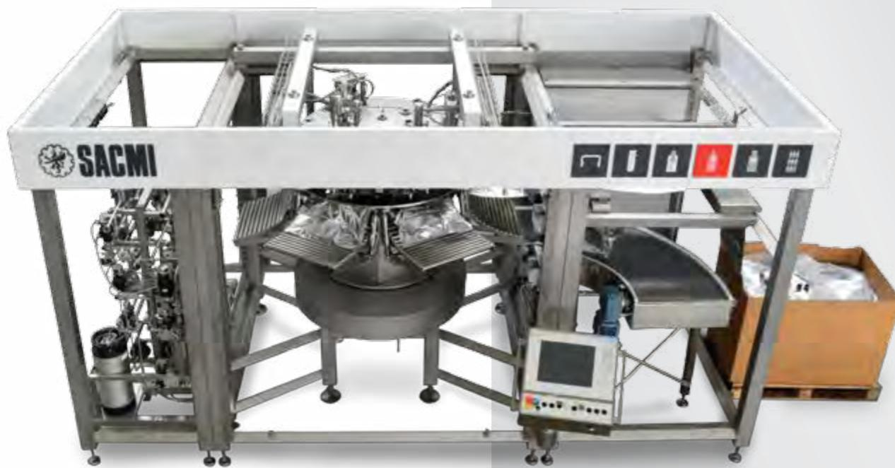
The filler is specially designed to automatically fill "pre-cut continuous module" or WEB type bags. Any type of spout may be used, even with a single guide spout, and may be placed in any position on the bag. A "size change over" kit is provided for each type of spout. All the most delicate operations that affect cap sterility such as uncapping, filling and capping take place in an aseptic chamber where the steady controlled flow of sterile air maintains a sterile environment at all times.
