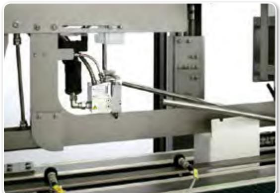
Automatic box closing machine with closing of the upper flaps by means of Hot Melt glue
