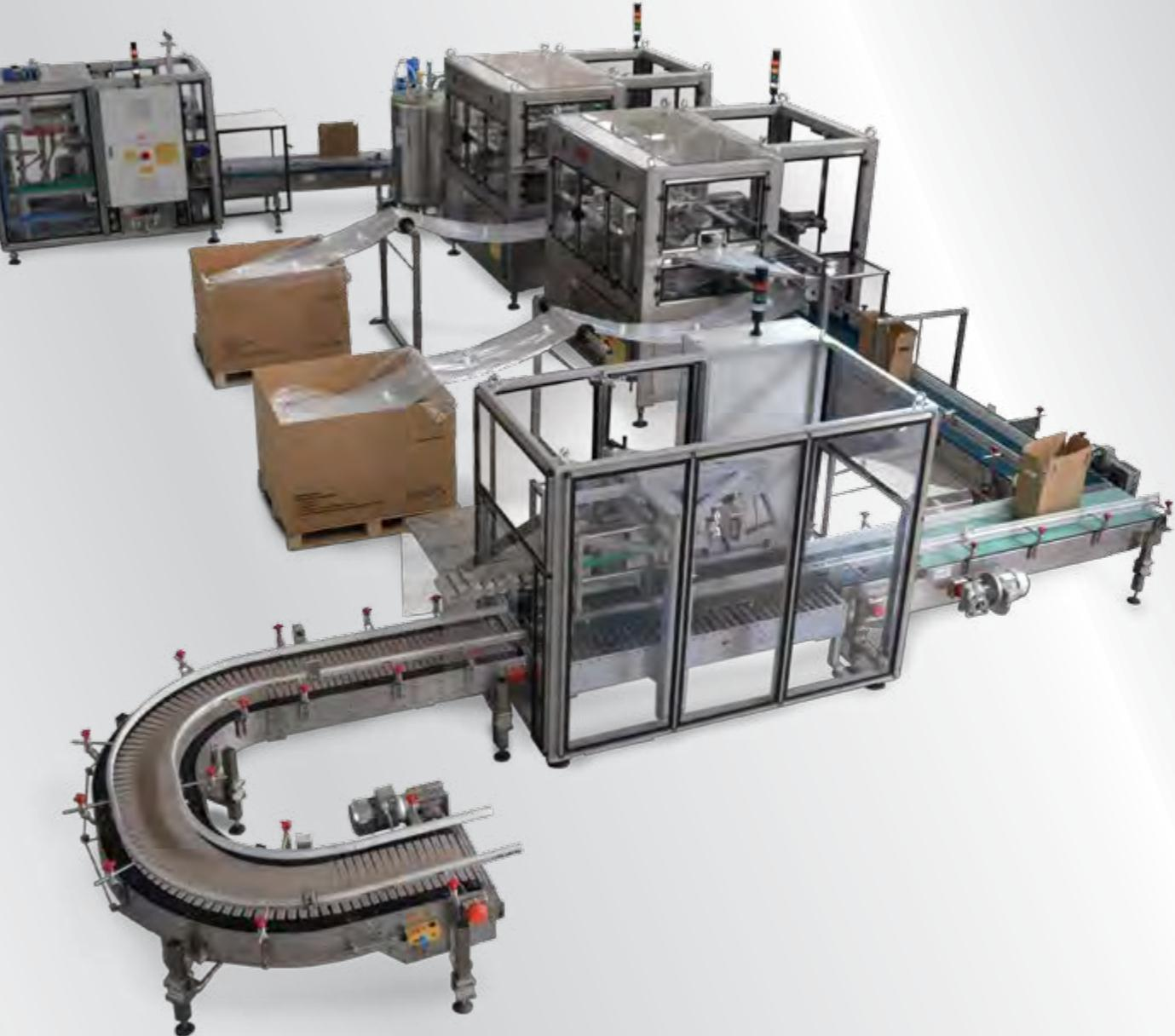
Completed packaging line composed of one case-former, by hot melt, number two filler model Linear, one case-closer by hot melt, including all the coupling conveyors
