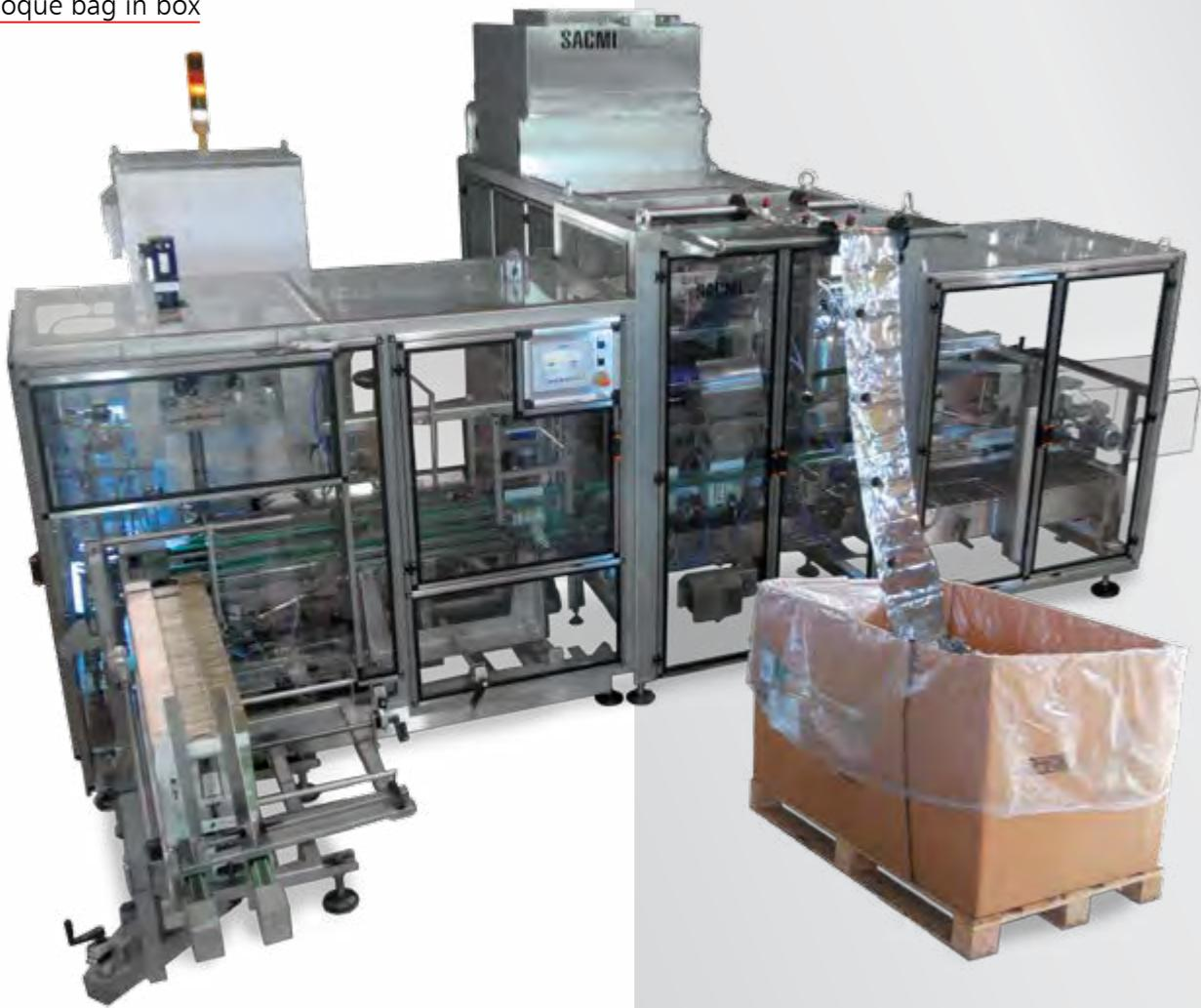
Monoblock suitable to square Bag in box cartons, to fill the bag and close the Bag in box automatically, by means of hot melt glue.
